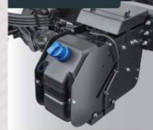
HDPE DEF Tank
